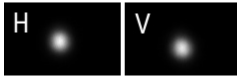
Figure 3.7: Spatial modes of the main output at different polarisations.
